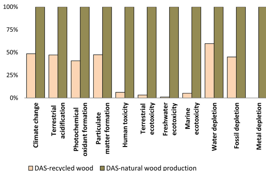
Fig. 5. Differences in impacts related to the use of recycled and natural wood materials to fill the reactive tanks. Results are normalized using the greatest value in each impact category. The use of recycled wood gives a reduction of more than 50% in almost all impact values, and even close to 100% for some categories.
